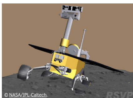
Figure 1. A computer-drawn picture showing how Spirit's wheels became stuck in soft material on Mars.
